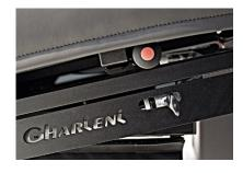
**NOTICE!** The additional lock <u>must</u> be released to adjust the armrests using the respective levers (s. chapter 10.7 ARMRESTS). Otherwise the construction and the mechanics of the armrests can be damaged permanently. RISK OF DAMAGE!
