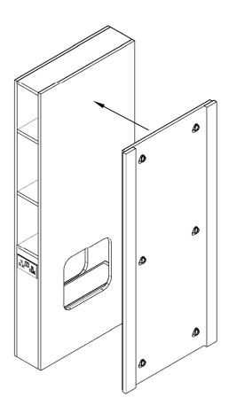
2. Fix Icon Back Board (A) to Island Column (E1) (no fixings supplied)
