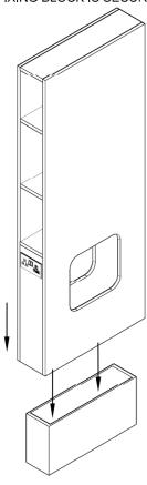
1. 2 person assembly process: Secure Floor Fixing Block (E2) to floor in required location (no fixings provided). Carefully lower Island Column (E1) over Floor Fixing Block. All electrics to be installed by a qualified electrician.
