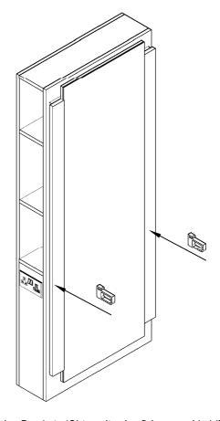
4. Fix Shelf Fixing Brackets (C) to unit using fixings provided (E).
