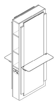
5. Insert shelf (D) into brackets and tighten from underside to secure in place.
