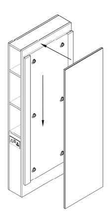
3. Carefully place Mirror Section (B) against Back Board (A), Ease down until the fixings meet and lock in place.
