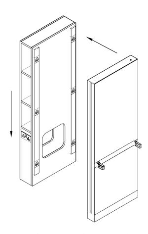
2. 2 person stage - Connect electrical / power cables before completing this procedure:
