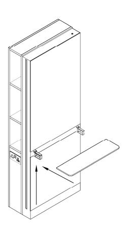
3. Unscrew (not fully) screws to bottom of shelf brackets to loosen. Carefully slide Glass Shelf (C) into shelf brackets. Fasten into place by re-tightening bracket screws.
